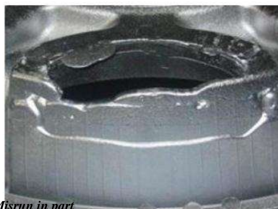
Fig Misrun in part
