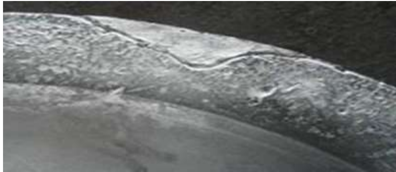
Fig Cold shut in part
