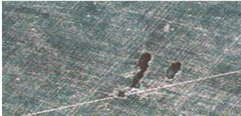
Fig Shrinkage Porosity
